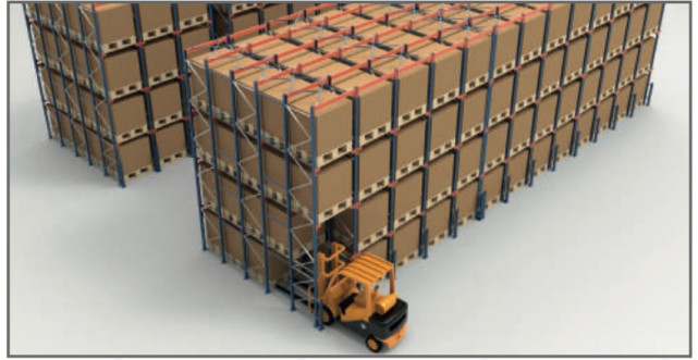
Drive-In Racking System
